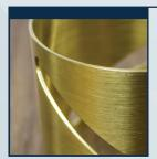
Walls should have a minimum width of 1/16" (1.5875mm). This is to avoid both chatter and the need to slow down machining speed.
