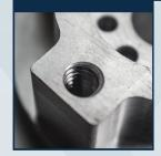
Utilize standard tap sizes such as 4-40 taps. Utilize standard fractional, number or letter drill sizes. Avoid very small holes and avoid threading more than 3x the hole's diameter.
