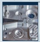
Especially useful for parts with deep pockets or multiple faces that require operations: design and machine as separate parts, then weld or bolt together.
