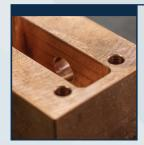
Assign numerical values to critical features and surfaces, and keep all other features as standard tolerance: +/- 0.005". Define a single datum, like the intersection of two sides, as a baseline.
