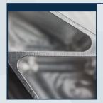
Use an inside corner radius with a depth-to-tool diameter ratio of 3:1 or less and avoid varying internal corner radii. Design lengths up to 4x their depth.
