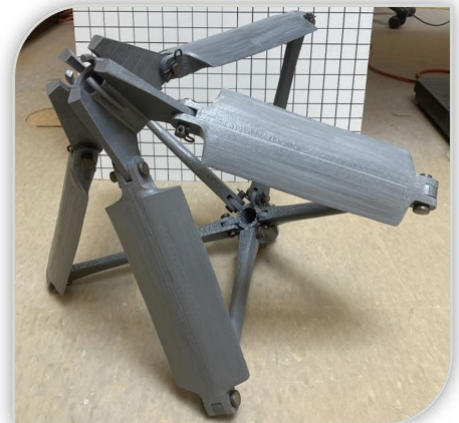
John Huntoon's Analytical Model of In-Situ Root-Inspired Ground Anchor Actuation and Pullout
