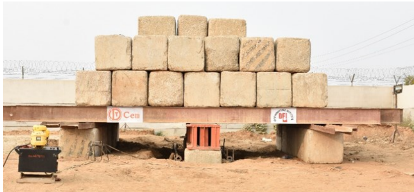
Figure 1: Typical loading platform for Kentledge test.
