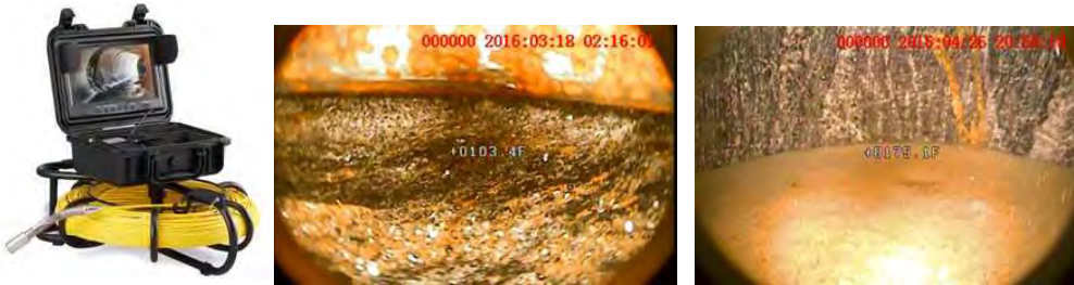
Fig.5: Down-hole Camera Equipment and Rock Socket Views
