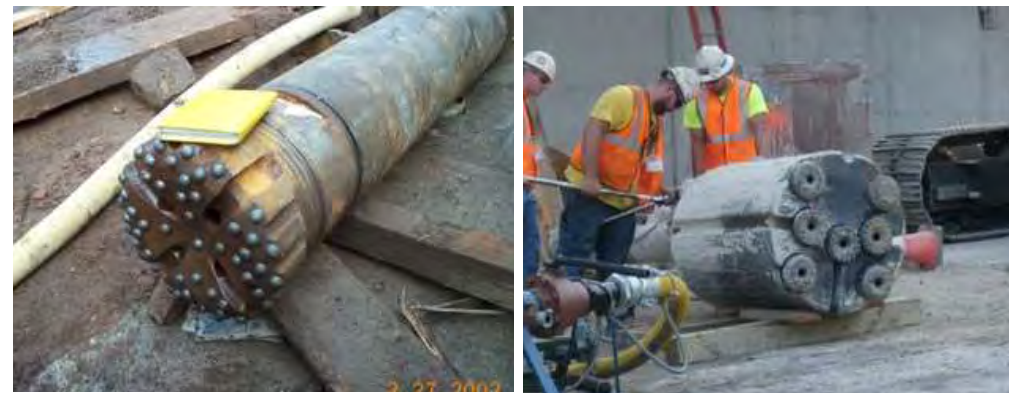
Fig. 4: Small and Large Diameter Down-the-hole Air Hammers
