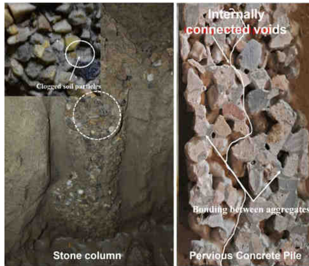
(Left) Fig. 2 Failed stone column post shake table testing under multiple dynamic loading at GEGH laboratory, CSIR CBRI, Roorkee (Right) Fig. 3 Inner core of pervious concrete
