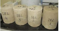
Fig. 2: Soil-Cement specimens moulded with different percentages of cement (Left); Fig. 3: Condition of specimens after completion of 12 cycles (Right)
