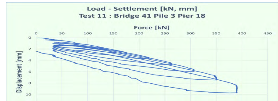
Fig. 3: Result of the static load test: the load settlement of one of the piles of bridge 41
