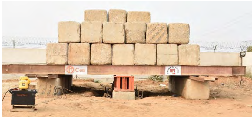
Figure 1: Typical loading platform for Kentledge test.
