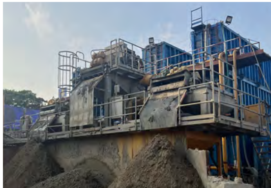
Fig. 3. Desanding plant (Pic Courtesy: Bauer Engineering India)
