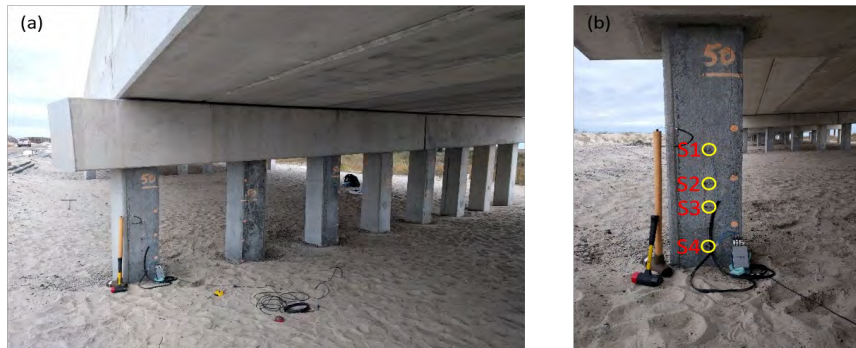
Fig 2: Prestressed concrete piles in North Carolina, USA (a) Site (b) Instrumented pile
