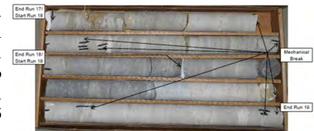
Fig 1b: Corresponding Photograph of recovered Dolostone Bedrock core
