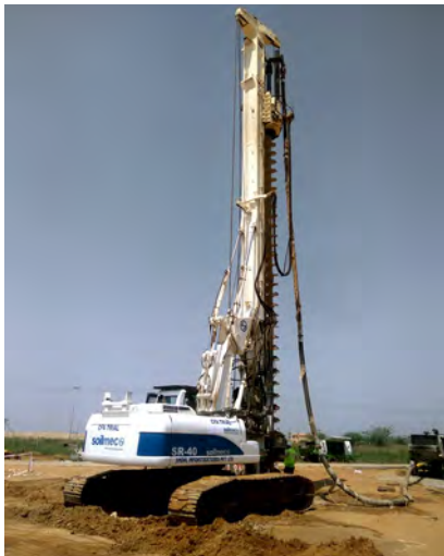
Fig. 4 CFA RIG- Courtesy - DFI India
