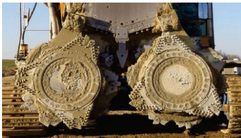
Figure 2: Mixing head for CSM with symmetric mixing wheels
