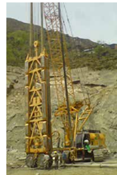
Fig. 6: Trench Cutter at a Dam Cut-off Wall Site
