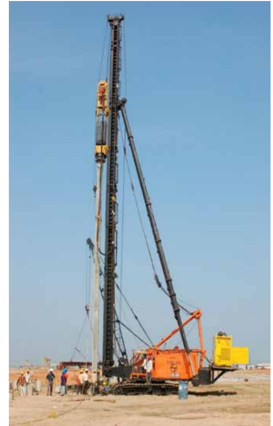
Fig. 1: Integrated Driven Piling Rig with Hydraulic Hammer
