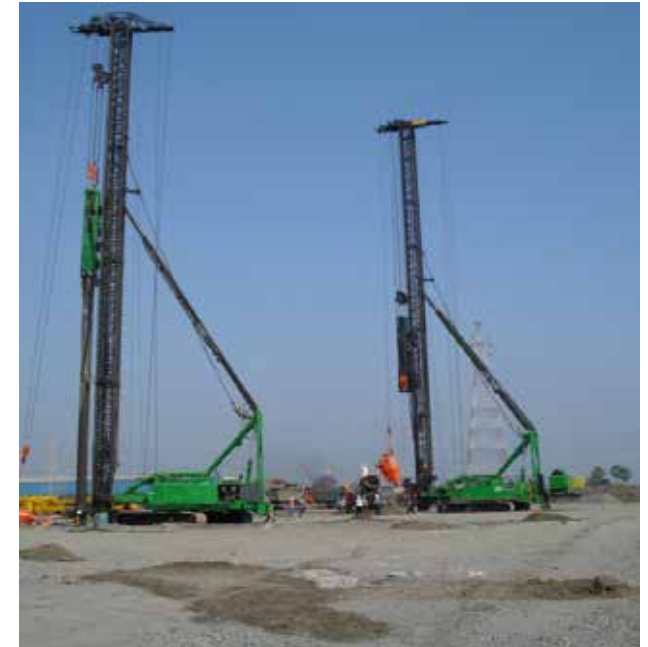
Fig. 3: Integrated Multipurpose Piling Rig with Hydraulic Hammer for Driven cast in situ Piles
