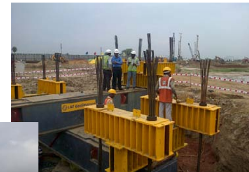
1200mm dia 40m deep piling on D&B mode, and capacity proven with instrumented load tests in Noida
