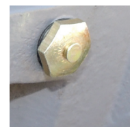
Grease pressure reliefs act to battle overgreasing
