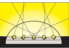
Patlite has created a revolutionary patented lighting design in which multiple LEDs project light across a broad peripheral area, ensuring equal intensity at the sides as well as the front. This design, with its side-projection technology, is a unique achievement in signal light design.
