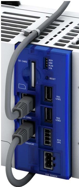
Fig. 1: Installation and fixing of the network cables
