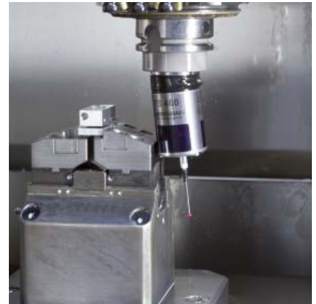
TS 460 with collision protection
