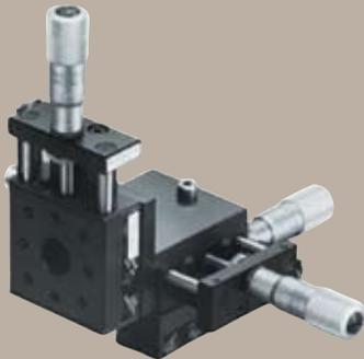
Parker Daedal precision linear stages provide controlled, precise point-to-point positioning along a linear axis. Stages are comprised of two basic components: a precision linear ball slide which serves as a linear bearing and guide, and a drive mechanism which accurately moves and positions the slide top along the linear axis.
