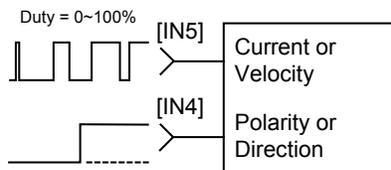
Another type of PWM input is the "50%" type. There is only one PWM signal that connects to [IN5]. The other digital input, [IN4], is not used in this mode. A 50% duty-cycle corresponds to a zero-current command in torque mode, or a zero-speed command in velocity mode.
