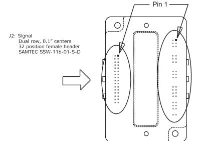
Drive viewed from above looking down on the pc board on which it is mounted. Pins and housing shapes are shown in phantom view.
