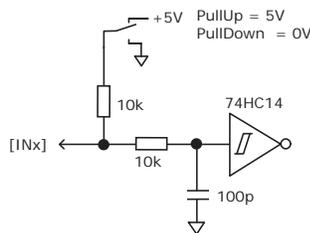
INPUTS WITH PROGRAMMABLE PULL UP/DOWN
