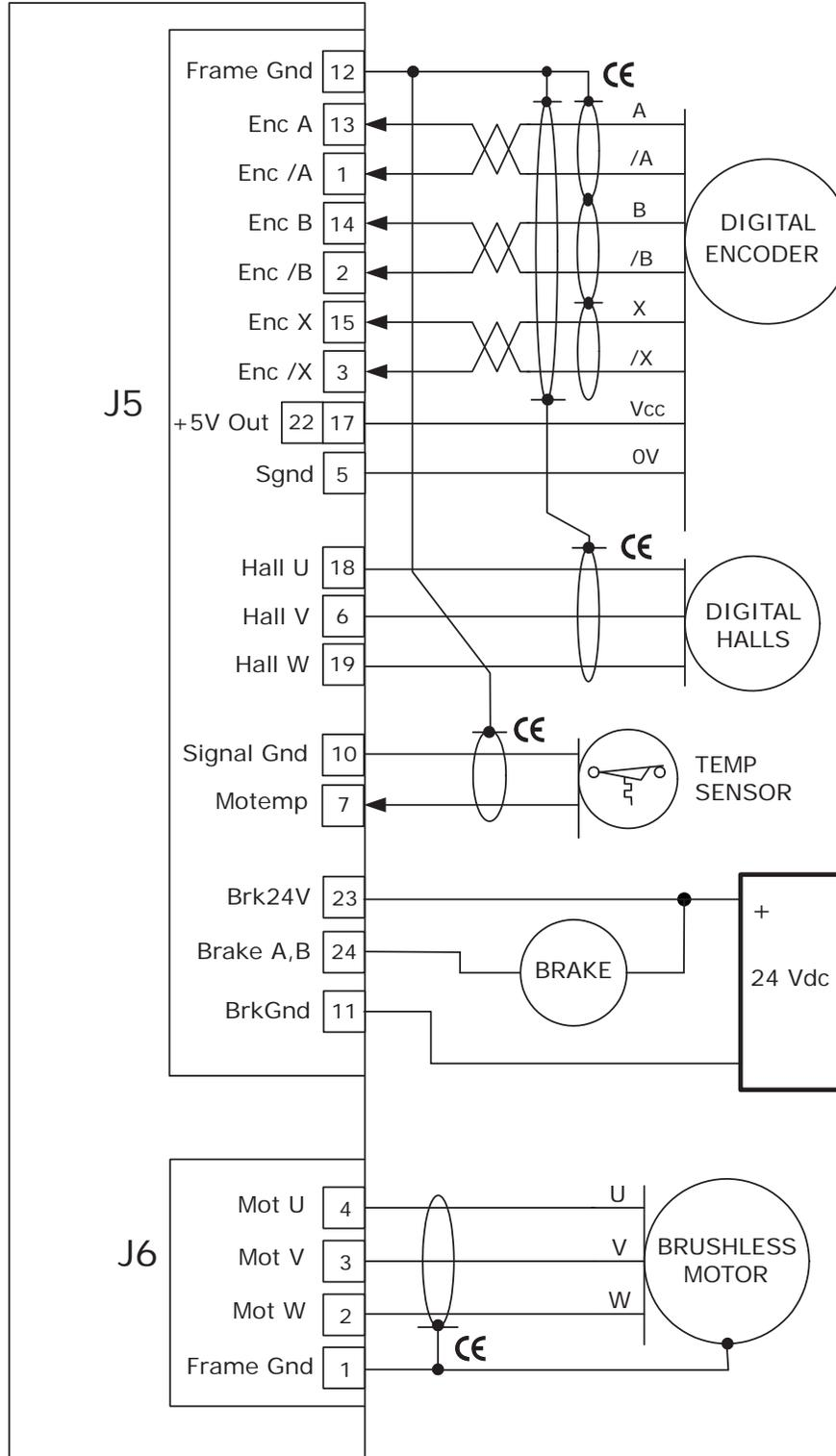
MOTOR CONNECTIONS FOR INCREMENTAL ANALOG (SIN/COS) ENCODERS
