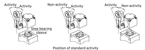
2. The rolling wheel could be installed at the inside of leverage
