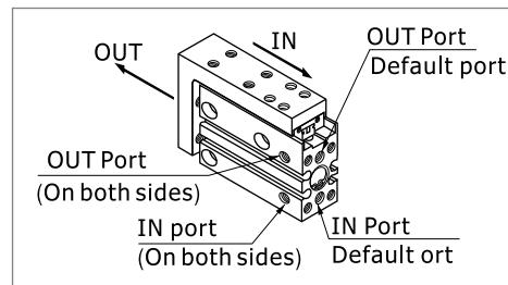
4. When the output of the compact slide will be directly applied to the table, it should be applied along the rod axis.
