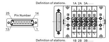
Note: Gauge number of cable connecting to D-Sub pin No.13(COM) must be≤22AWG
