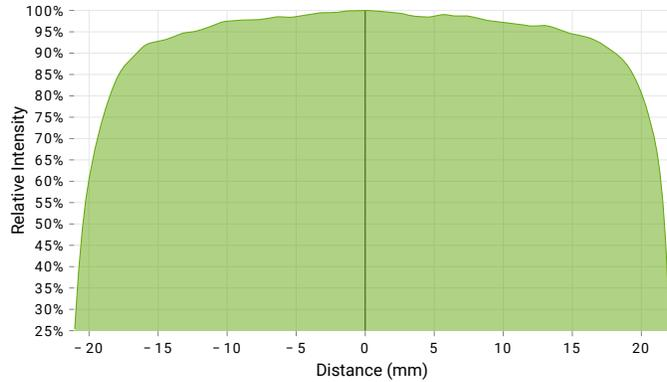
The BL245 Series provides a highly uniform output across its emitting window with an edge effect of only 18.4mm, and a uniformity of +/- 10% within the optical area.
