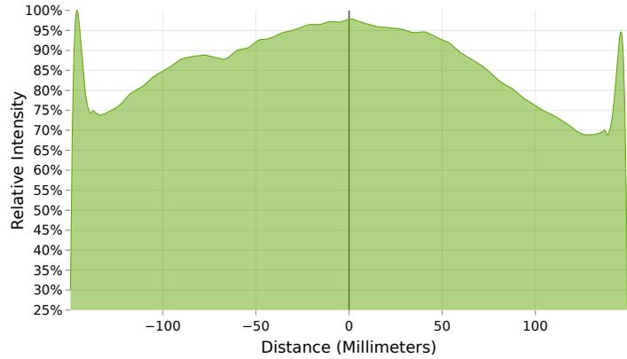
The BX2 Series' uniformity is dependent on the size configured. Models with an emitting length greater than 200mm have a uniformity of +/- 15%, while those with an emitting length less than 200mm achieve +/- 10% uniformity within the optical area.
