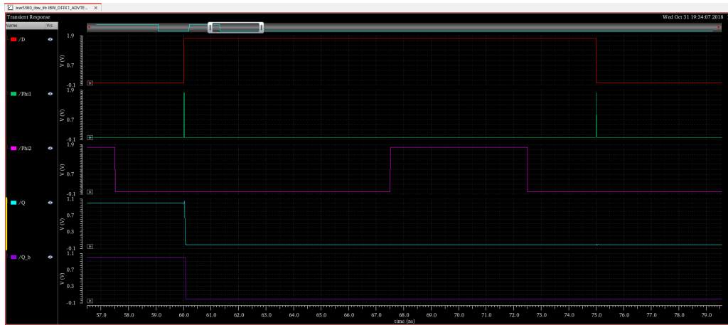
Figure 3.12: Phi1 Minimum Pulse Width Waveform
