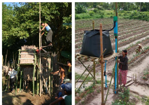
Figure 4. Elevated ordinary treadle pump (left) and new Sin Pauq pump with Proximity drip system (right).
