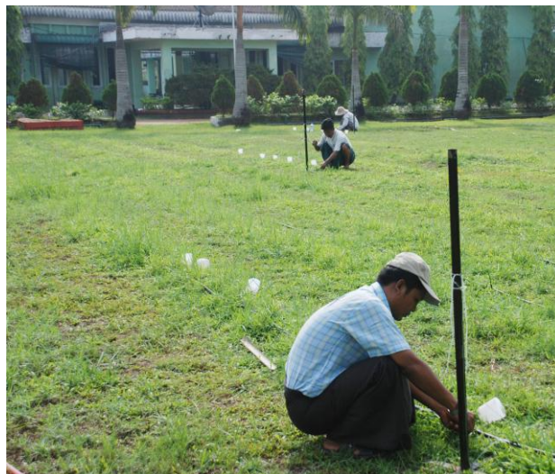
Figure 3. Manometers and catch cans used in drip system performance testing, 2009-10.
