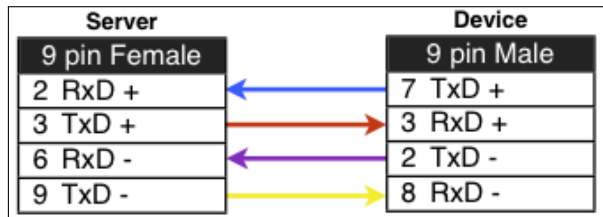
FIGURE 2.33: Quatech RS-422 cable
