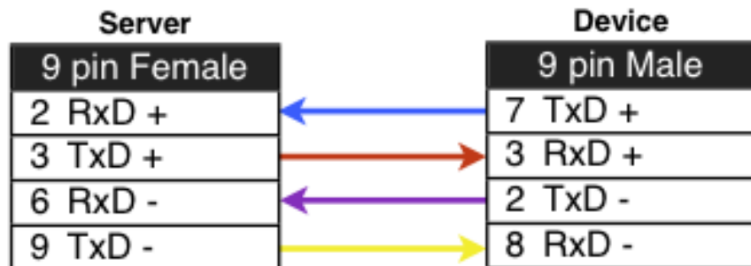
FIGURE 2.50: Quatech RS-422 cable
