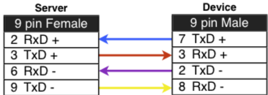
FIGURE 2.39: Quatech RS-422 cable
