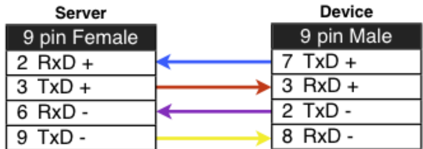
FIGURE 2.45: Quatech RS-422 cable
