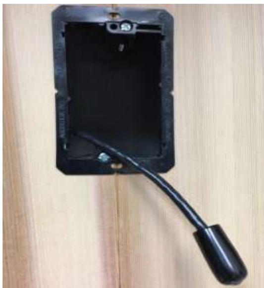
3. With the boot removed, insert the male RJ-10 connector into the female receptacle of the External Switch, as shown.
