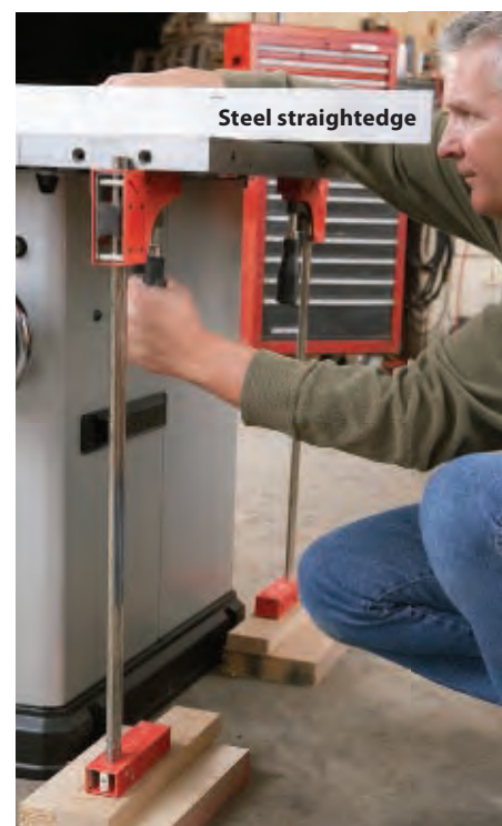
6. To remove sagging, changing a clamp to spreader mode lets you microadjust the wing height. Parallel-jaw clamps work great for this.
