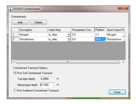
**Note:** The base output file column specifies the location of the output files that will be generated for each contaminant. These output files will be written in the same folder where your project files are located (in this case | GSSHA Distributed Hydrologic modelings | Personal | Contaminants |)
