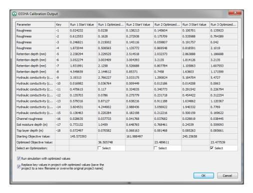
If using the SLM local optimization method, only a single set of optimized values will be visible. If using the MLSL method described above, there will be multiple sets of optimized values. Select the desired set of optimized values from the dialog.
