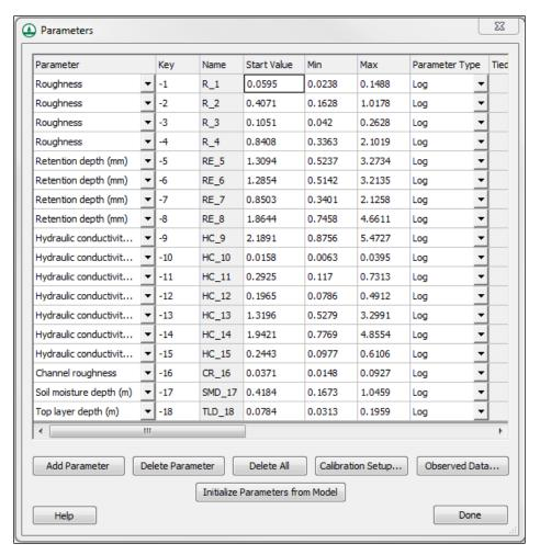
5. Enter the Start Value, Min and Max values as shown in the figure above by copying and pasting the values from the file \Calibration\Automated\InitialParams.txt, found in the data files for this tutorial. Guidance for starting parameter estimates can be found on http://gsshawiki.com.
