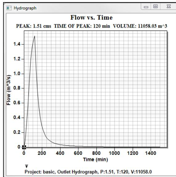
Figure 3 Runoff hydrograph
