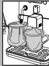
20 Place an empty container under the steam wand and another one under the dispensing spout.
