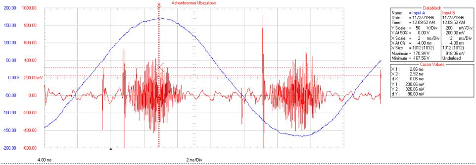
The waveform was collected with a Fluke 199 Scopemeter at the Kevin Ashenbrenner home. Channel A was connected to a 120V receptacle. Channel B was connected at the same potential except through the Graham ubiquitous filter (removes the 60 cycle). The area between the cursors represents a frequency of 16.6 kHz. The high frequency is riding on the utility supplied 60 cycle waveform.
