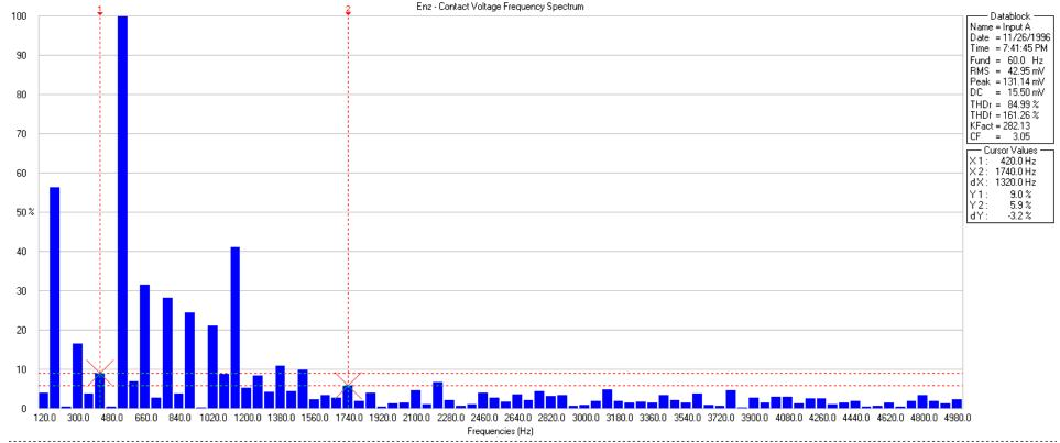
The above frequency spectrum is of a waveform collected between the sink and floor (contact Voltage) at the Dave and Rosemary Enz home near Denmark, WI.
