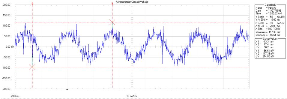
The waveform was collected with a Fluke 199 Scopemeter at the Kevin Ashenbrenner home. The leads were connected between the kitchen sink and an EKG patch placed on the floor. (Contact Voltage) Assuming a person has an impedance of 500 Ohms, the contact current would be 428 micro amperes or more than 23 times the current the NIEHS states is relevant to cancer.
