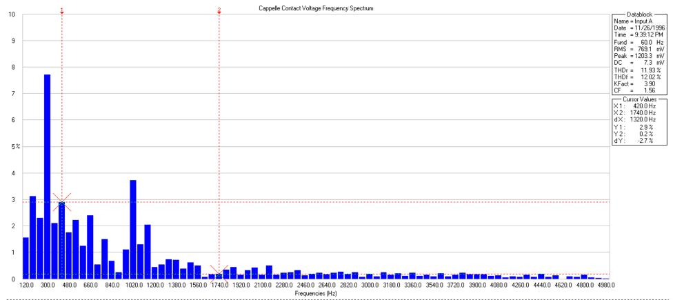
The above frequency spectrum is of a waveform collected between the sink and floor (contact Voltage) at the Cappelle home near Denmark, WI.
