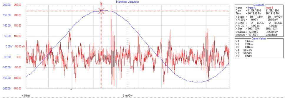
The waveform was collected with a Fluke 199 Scopemeter at the Mark and Tammy Brantmeier home. Channel A was connected to a 120V receptacle. Channel B was connected at the same potential except through the Graham ubiquitous filter (removes the 60 cycle). The area between the cursors represents a frequency of 16.6 kHz. The high frequency is riding on the utility supplied 60 cycle waveform.
