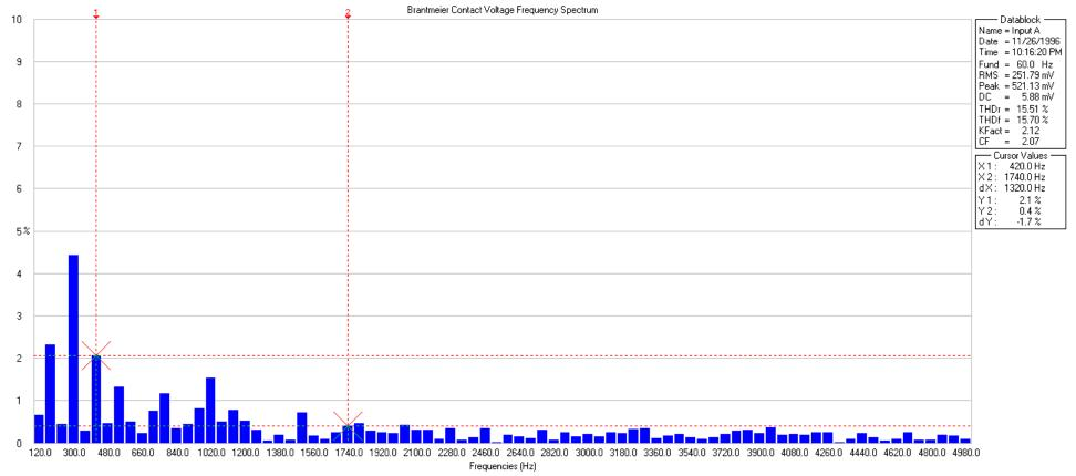
The above frequency spectrum is of a waveform collected between the sink and floor (contact Voltage) at the Brantmeier home near Denmark, WI.
