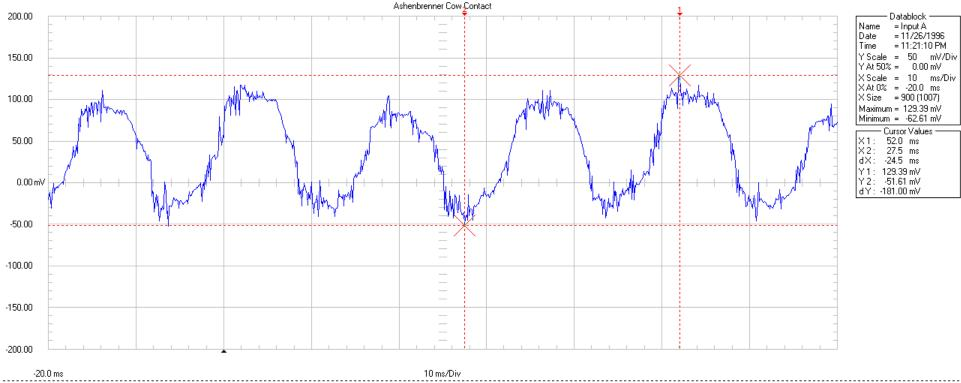
The waveform was collected with a Fluke 199 Scopemeter at the Kevin Ashenbrenner farm. Leads were connected between a 19 square inch stainless steel plate and the water pipe (cow contact). The voltage displayed on the above waveform is 181 mV.
