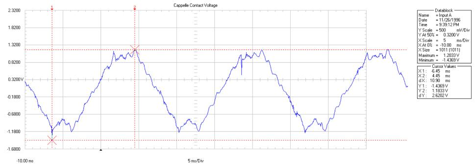
The waveform was collected with a Fluke 199 Scopemeter at the Darrel and Sarah Cappelle home. The leads were connected between the kitchen sink and an EKG patch placed on the floor. (Contact Voltage) Assuming a person has an impedance of 500 Ohms, the contact current would be 5,240 micro amperes or more than 291 times the current the NIEHS states is relevant to cancer.
