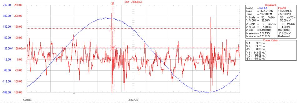
The waveform was collected with a Fluke 199 Scopemeter at the Dave and Rosemary Enz home. Channel A was connected to a 120V receptacle. Channel B was connected at the same potential except through the Graham ubiquitous filter (removes the 60 cycle). The area between the cursors represents a frequency of 12.5 kHz. The high frequency is riding on the utility supplied 60 cycle waveform.
