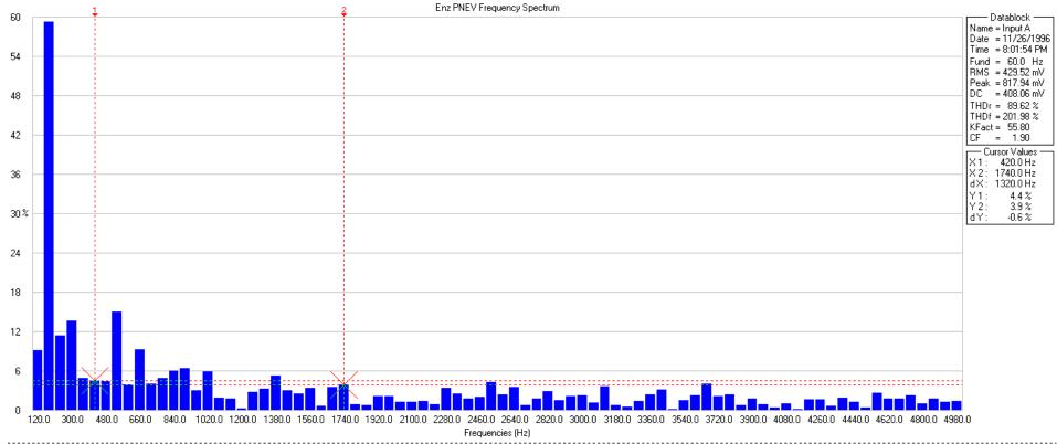
The above frequency spectrum is of a waveform collected at primary neutral to earth voltage at the transformer down ground across the road from the Dave and Rosemary Enz home near Denmark, WI.
