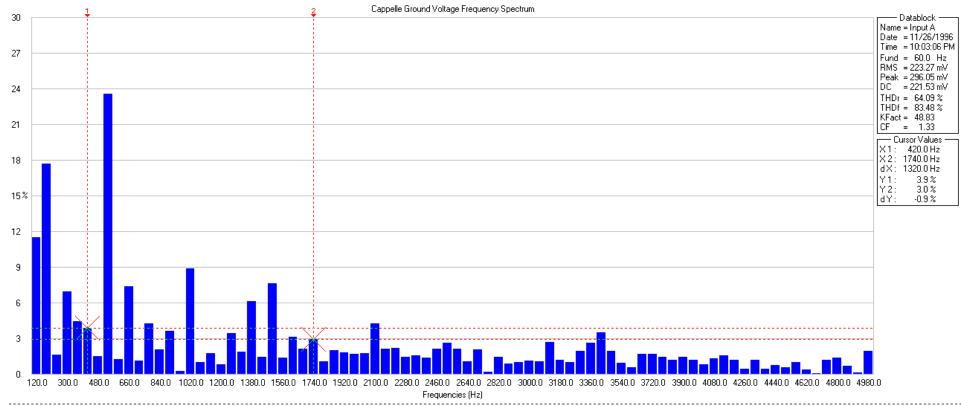
The above frequency spectrum is of a waveform collected between two remote ground rods in the yard of the Darrel and Sarah Cappelle home near Denmark, WI.
