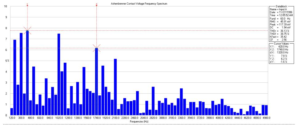
The above frequency spectrum is of a waveform collected between the sink and floor (contact Voltage) at the Kevin Ashenbrenner home near Denmark, WI.
