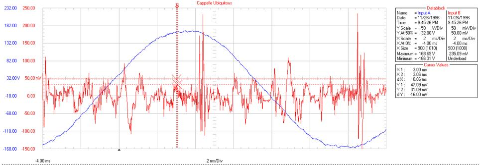
The waveform was collected with a Fluke 199 Scopemeter at the Darrel and Sarah Cappelle home. Channel A was connected to a 120V receptacle. Chan nelB was connected at the same potential except through the Graham ubiquitous filter (removes the 60 cycle). The area between the cursors represents a frequency of 16.60kHz. The high frequency is riding on the utility supplied 60 cycle waveform.
