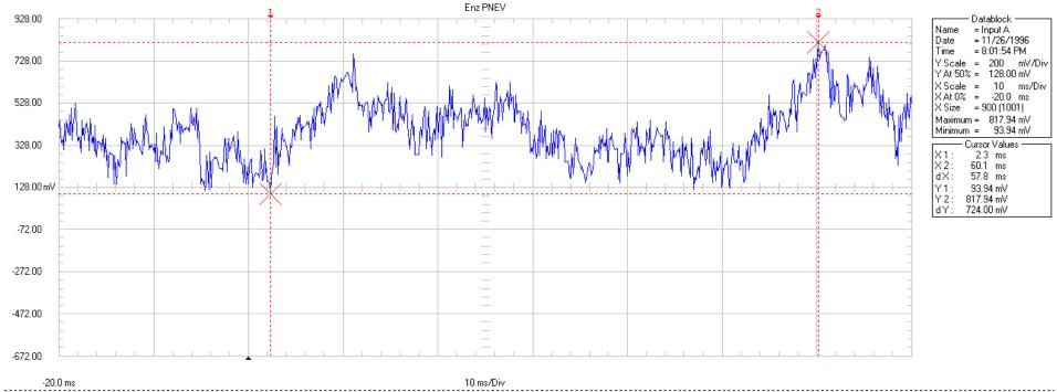
The distorted waveform was measured with a Fluke 199 Scopemeter at PNEV at the transformer down ground across the road from the Enz home near Denmark, WI. One lead was connected to the utlityprimary down ground and the other to a remote ground rod. The windturbines were running in close proximity to the measurement points.
