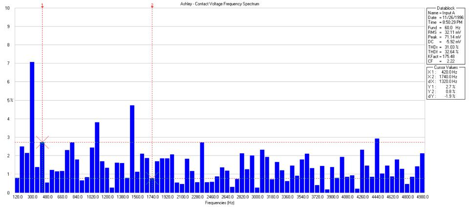
The above frequency spectrum is of a waveform collected between the sink and floor (contact Voltage) at the Ashley home near Denmark, WI.
