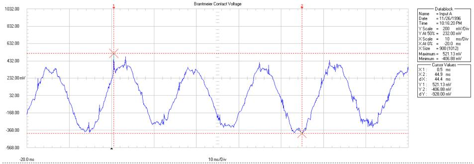
The waveform was collected with a Fluke 199 Scopemeter at the Mark and Tammy Brantmeier home. The leads were connected between the kitchen sink and an EKG patch placed on the floor. (Contact Voltage) Assuming a person has an impedance of 500 Ohms, the contact current would be 1856 micro amperes or more than 103 times the current the NIEHS states is relevant to cancer.
