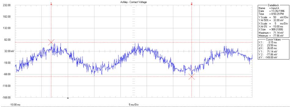
The waveform was collected with a Fluke 199 Scopemeter at the Ashley home. The leads were connected between the kitchen sink and an EKG patch placed on the floor. (Contact Voltage) Assuming a person has an impedance of 500 Ohms, the contact current would be 298 micro amperes or more than 16 times the current the NIEHS states is relevant to cancer.
