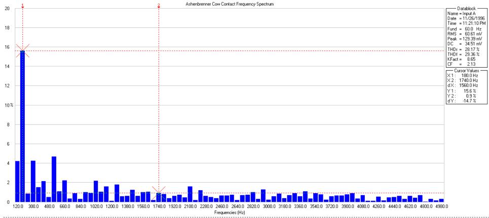
The frequency specrtum is of the cow a cow contact voltage waveform collected in the barn of Kevin Ashenbrenner, near Denmark WI.
