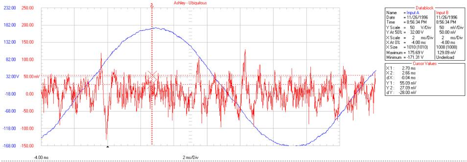
The waveform was collected with a Fluke 199 Scopemeter at the Ashley home. Channel A was connected to a 120V receptacle. Channel B was connected to the same potential except through a Graham ubiquitous filter (removes the 60 cycle). The area between the cursors represents a frequency of 25 kHz. The high frequency is riding on the utility supplied 60 cycle waveform.
