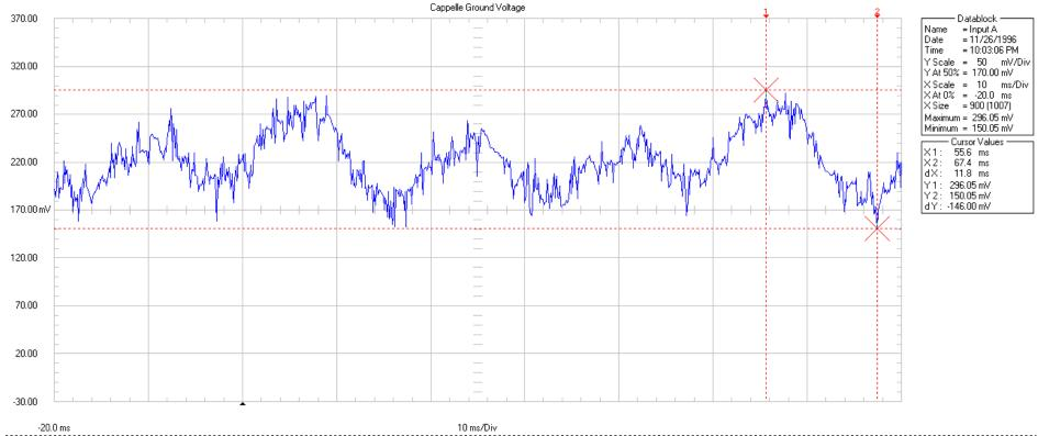
The distorted waveform was measured with a Fluke 199 Scopemeter. The leads were connected between two remote ground rods in the yard of Darrel and Sarah Cappelle.
