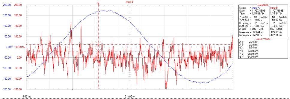
The waveform was collected with a Fluke 199 Scopemeter at the Jean and Larry Tenor home. Channel A was connected to a 120V receptacle. Channel B was connected at the same potential except through the Graham ubiquitous filter (removes the 60 cycle). The area between the cursors represents a frequency of 25kHz. The high frequency is riding on the utility supplied 60 cycle waveform.
