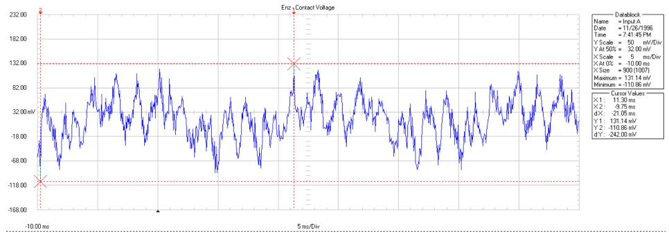
The waveform was collected with a Fluke 199 Scopemeter at the Dave and Rosemary Enz home. The leads were connected between the kitchen sink and an EKG patch placed on the floor. (Contact Voltage) Assuming a person has an impedance of 500 Ohms, the contact current would be 484 micro amperes or more than 26 times the current the NIEHS states is relevant to cancer.
