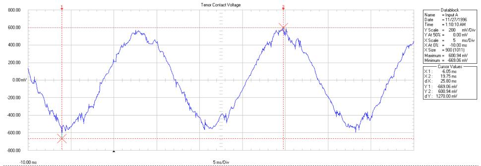
The waveform was collected with a Fluke 199 Scopemeter at the Jean and Larry Tenor home. The leads were connected between the kitchen sink and an EKG patch placed on the floor. (Contact Voltage) Assuming a person has an impedance of 500 Ohms, the contact current would be 2,540 micro amperes or more than 141 times the current the NIEHS states is relevant to cancer.
