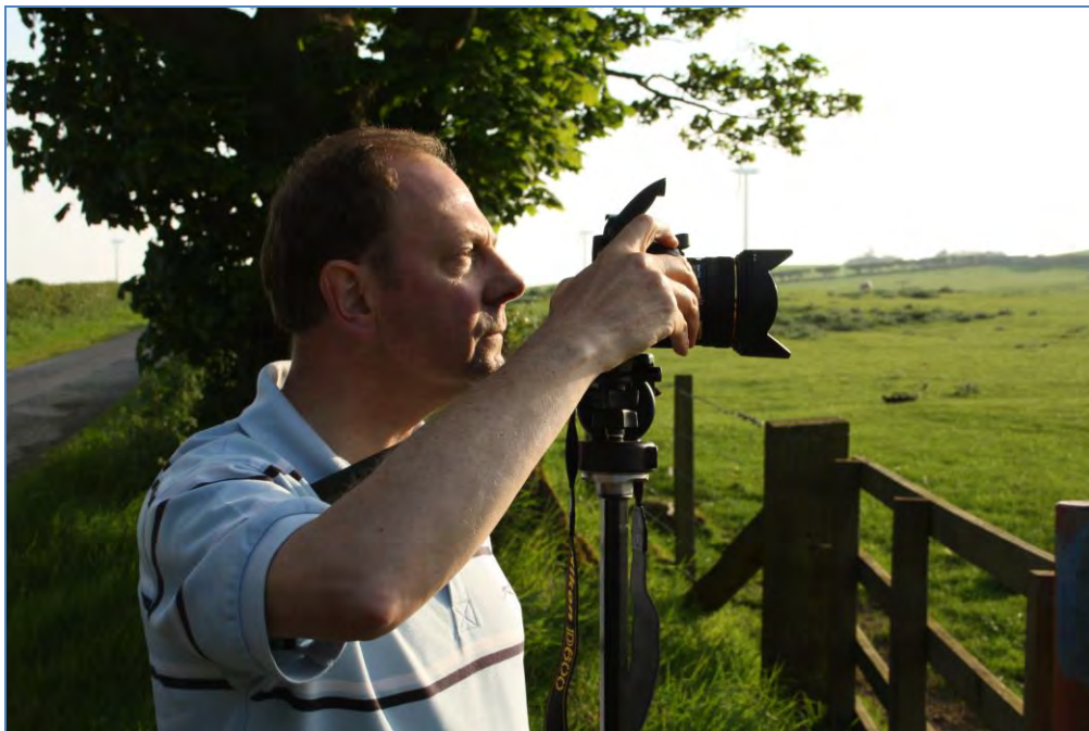
Figure 3: Reflecting best practice, using full frame DSLR camera with fixed 50mm lens with levelling tripod at North Charlton, Wandylaw Wind Farm.
