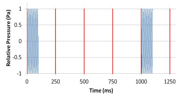
FIGURE 2d. This figure shows a notional 1000 Hz wave form present for the first 100 ms of each second. We term this notional because the actual frequency rate portrayed is about 100 Hz rather than 1000 Hz, which would just show as a solid block, and not as a sine wave. Red lines mark each 250 ms interval.
