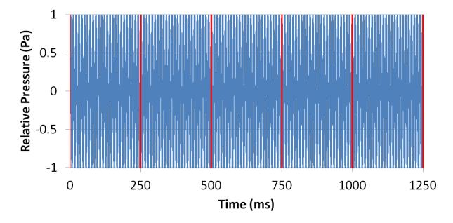
FIGURE 2a. This figure notionally shows a 1000 Hz sine wave with a continuous waveform. Since this figure cannot be meaningfully analyzed in this form, the following 1000 Hz figures are notional 1000 Hz figures, because the actual frequency rate portrayed is about 100 Hz rather than 1000 Hz, which would just appear as a solid block. Red lines mark each 250 ms interval.
