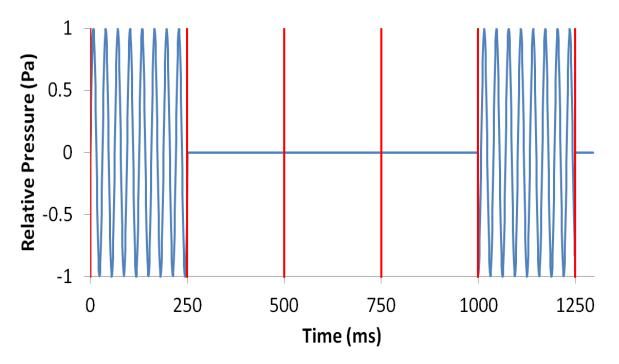
FIGURE 3b. This figure shows a 31.5 Hz wave form present for the first 250 ms of each second. Red lines mark each 250 ms interval.
