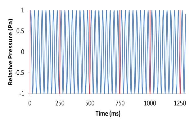
FIGURE 3a. This figure shows a 31.5 Hz continuous waveform. Red lines mark each 250 ms interval.
