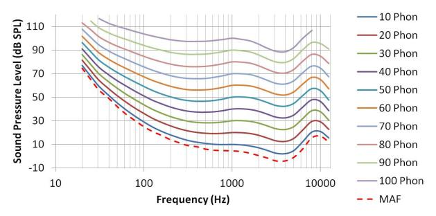
**FIGURE 1.** This figure shows the equal-loudness contours in accordance with ISO 226:1987. Note that at low frequencies the contours come together, and for most of the 20 to 30 Hz range, a 10 dB change in sound pressure level corresponds to a 20 phon change. NOTE: the 1987 contours are used because the 2003 contours are only defined from 20 phon to 90 phon, and they do not include the minimum audible field (MAF).
