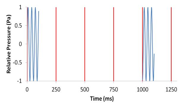
FIGURE 3c. This figure shows a 31.5 Hz wave form present for the first 100 ms of each second. Red lines mark each 250 ms interval.
