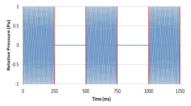
FIGURE 2b. This figure shows a notional 1000 Hz wave form turning on and off every 250 ms (we term this notional because the actual frequency rate portrayed is about 100 Hz rather than 1000 Hz, which would just show as a solid block, and not as a sine wave). Red lines mark each 250 ms interval.
