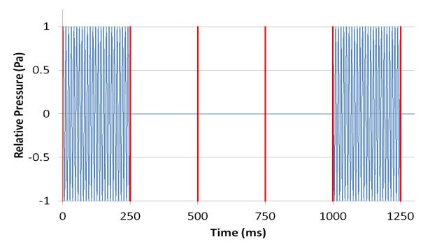
FIGURE 2c. This figure shows a notional 1000 Hz wave form present for the first 250 ms of each second. We term this notional because the actual frequency rate portrayed is about 100 Hz rather than 1000 Hz, which would just show as a solid block, and not as a sine wave. Red lines mark each 250 ms interval.
