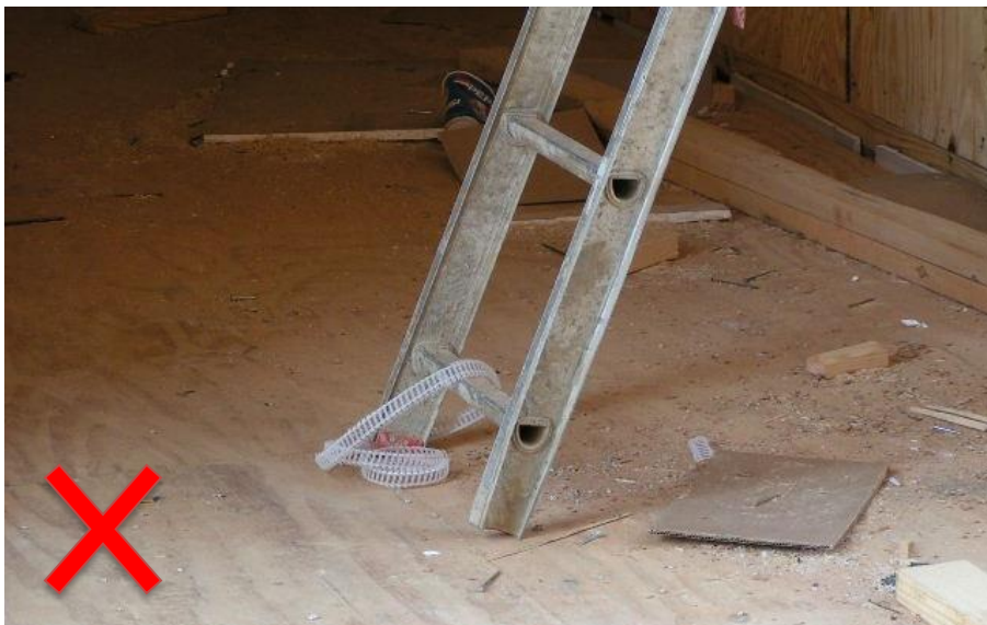
Extension ladder missing foot assembly and foot pads. This appears to be the top portion of an extension ladder that has been taken apart.
