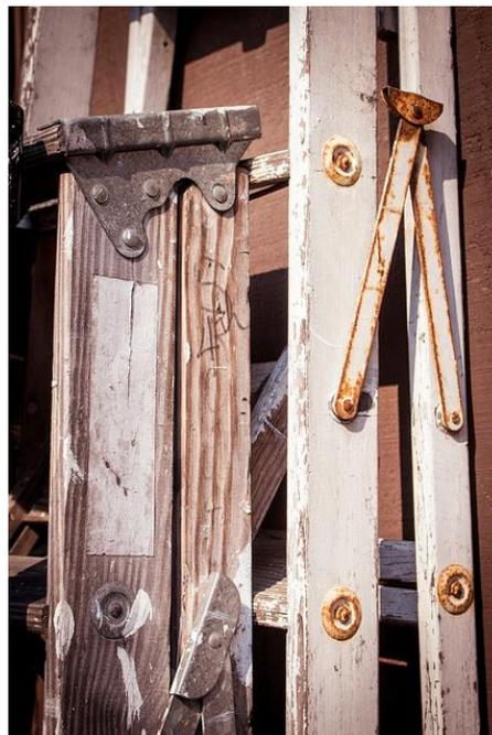
Close up view of wooden ladder rails and spreaders. Note: rails and spreaders appear to be worn and rusted and should be removed from service and tagged "Do Not Use". (\*4)
