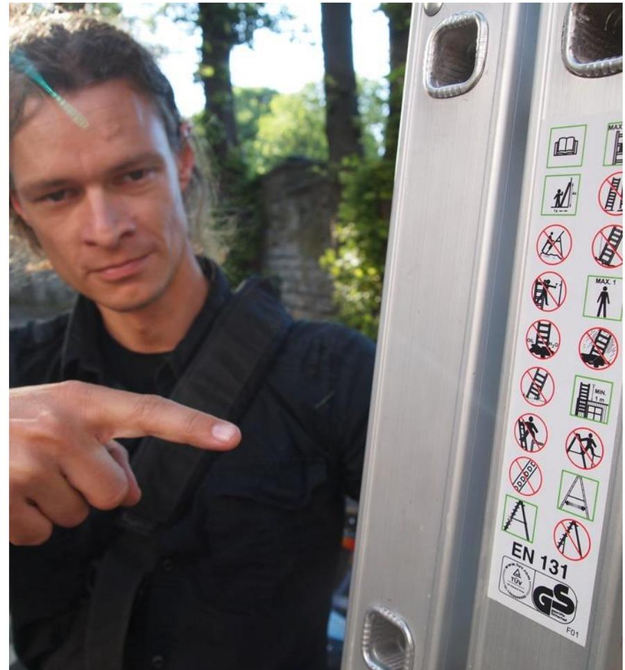
*Individual pointing to the manufacturer's safety labels and warnings on the ladder. Ladder inspections should include making sure that labels are readable and haven't been painted over or damaged. (\*1)*
