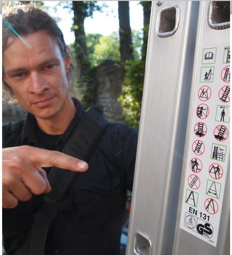
*Manufacturer's safety labels and warnings on the ladder. Ladder inspections should include making sure that labels are readable and haven't been painted over or damaged. (\*1)*
