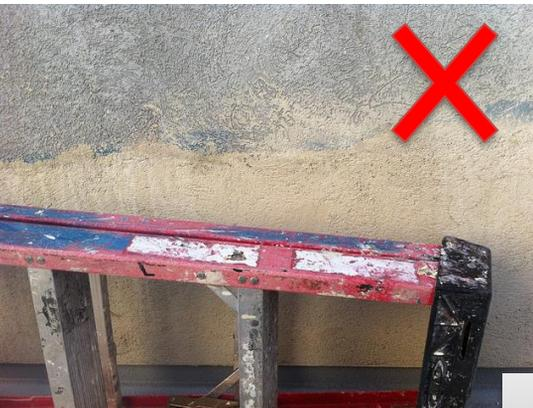
*Paint and grime covering the labels and steps of this ladder. It should be removed from service and cleaned to avoid a potential safety hazard. (\*8)*
