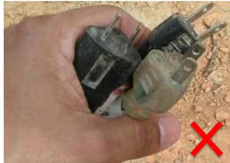
*Never use extension cords that have broken or missing ground pins!*
