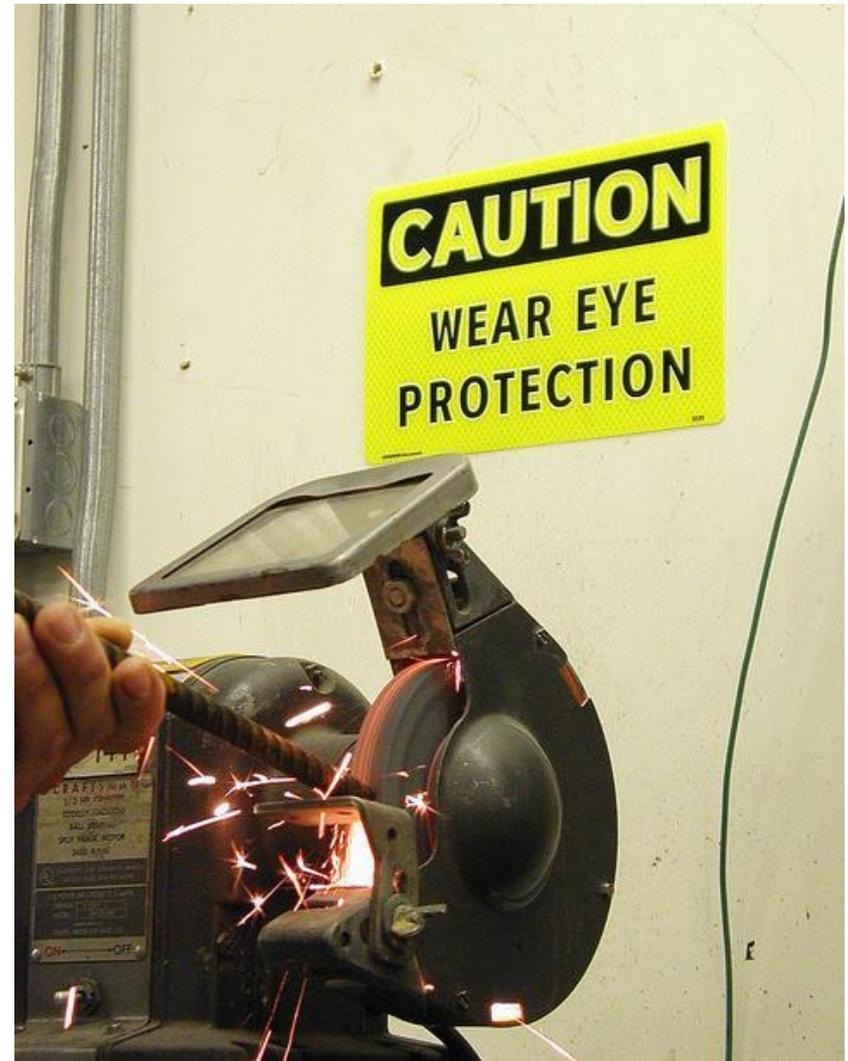
*Impact hazards can be created by grinding or cutting tools such as the bench grinder above. (\*3)*
