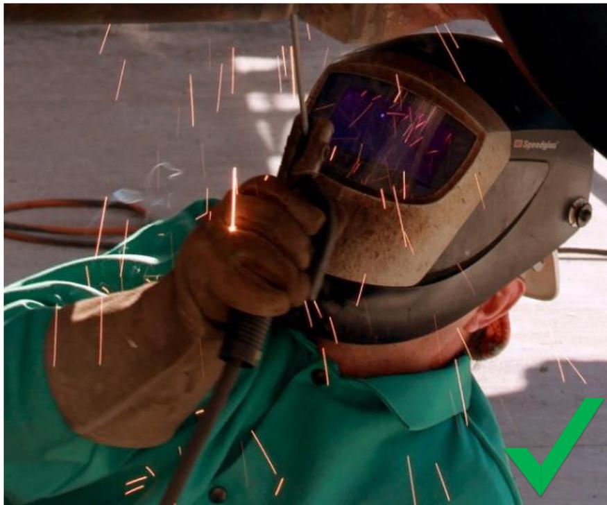
Worker properly welding with protective eye/face equipment. (\*4)
