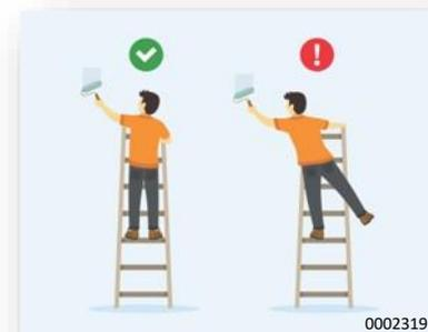
**OSHA Standard 1926.1053(b)(21)** *Each employee shall use at least one hand to grasp the ladder when progressing up and/or down the ladder.*
