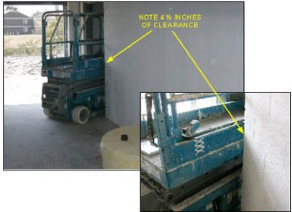
Image from a fatality investigation where a 42-year-old part-time laborer was killed when the scissor lift he was operating elevated and pinned him against the header of an interior doorway. NIOSH In-house FACE Report 2003-01 (*6)
