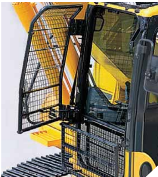
Cab front full height guard level 1 (ISO 10262)
